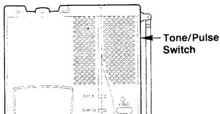
Set the TONE/PULSE switch located on the side of the base unit for the type of service you have (tone or pulse). If you are not sure which type of service you have, do this simple test.
