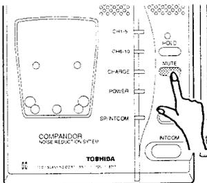
Pressing the MUTE button turns off the microphone during a telephone conversation at the speakerphone and the intercom so that you may speak to someone in the room with you without the caller overhearing. The SP/INTCOM LED will blink in this mute mode. Press the SPEAKERPHONE button or MUTE button again to resume normal conversation.
