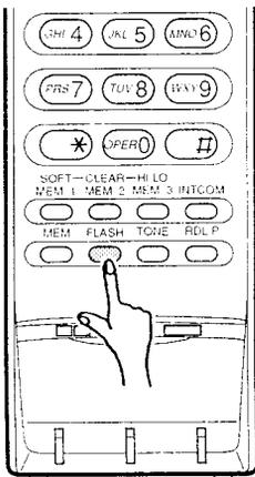
The FLASH button is used to send a timed hookflash on the telephone line for accessing services such as call waiting, etc. (Call Waiting is a telephone company service).
