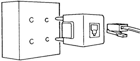
An adaptor (not included) is required. The adaptor plugs into the 4-prong jack and the phone's modular plug plugs into the adaptor.
