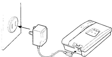
Connect the plug at the end of the AC adaptor to a standard 120V AC outlet and the other end to the rear of the base unit.
