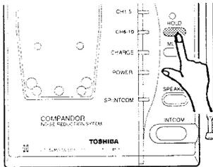
Once the speakerphone on the base unit has been activated, you may place a call on hold by pressing the HOLD button on the base unit. The HOLD LED will light and the SP/INTCOM LED will be turned off. To resume your conversation, simply press the SPEAKERPHONE button or HOLD button again.
