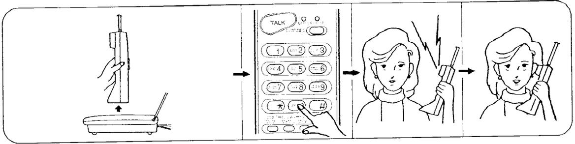
Lift the handset from the base unit, and press the TALK button. The CHANNEL LED lights.
