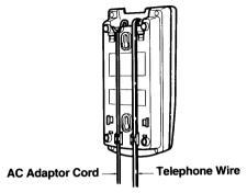
Place the base's keyhole slots over the two screws and gently push down on the base unit to lock it into place.
