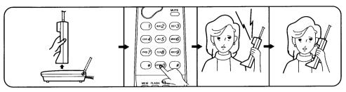
Lift the handset from the base unit, and press the TALK button. The TALK/BATT. LOW LED lights.
