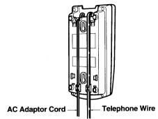
Place the base's keyhole slots over the two screws and gently push down on the base unit to lock it into place.
