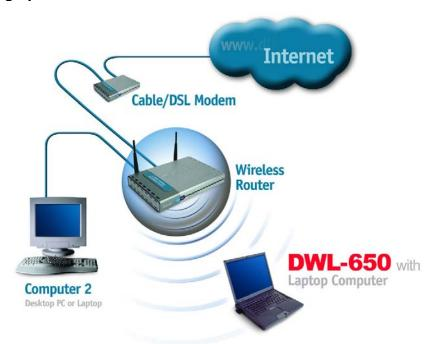
Please remember that **D-Link Air** wireless devices are pre-configured to connect together, right out of the box, with the default settings.
