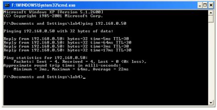
Go to **Start** > **Run** > type **cmd**. A window similar to this will appear. Type **ping xxx.xxx.xxx.xxx**, where **xxx** is the **IP address** of the Wireless Router or Access Point.
