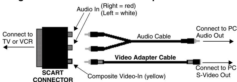
The SCART connector supports only the Composite video format, which means you will have to use the S-Video-to-Composite Video Adapter Cable. The above illustration shows how to connect your PC to a European TV using the SCART. If your European TV **does** support S-Video input, you should use an S-Video cable (available in most consumer electronic stores) rather than the SCART connector.
