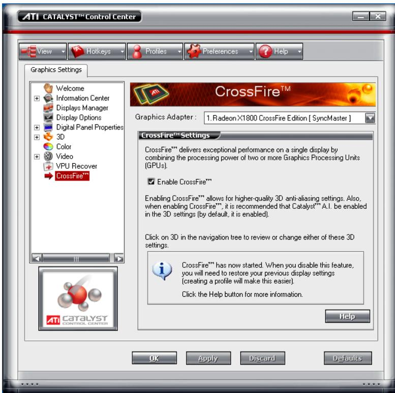
To access and enable CrossFire™ in Catalyst™ Control Center, do the following:
