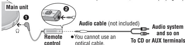
When connecting the unit to other equipment, set the volume level between 10 to 15, then use the volume control on the other equipment to adjust the volume.
