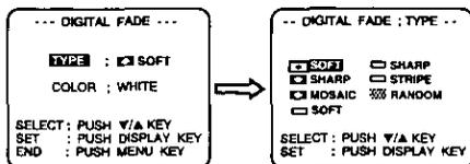
**4** Press **DISPLAY** for **DIGITAL FADE** menu. Press **DOWN ▼** to select **COLOR**. Press **DISPLAY** for **COLOR** menu. Press **UP ▲** or **DOWN ▼** to select from 8 colors.
