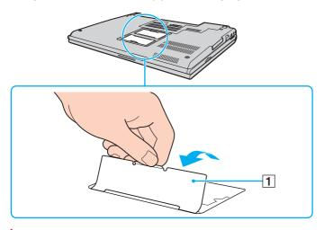
The inflation sheet is equipped for module protection. Do not pull it too hard to damage the sheet.
