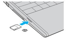
Be sure to hold the Memory Stick media with the arrow pointing in the correct direction as you insert it into the slot. To avoid damaging the computer or the Memory Stick media, do not force the Memory Stick media into the slot if it does not insert smoothly.
