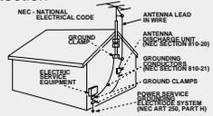
information regarding proper grounding of the mast and supporting structure, grounding of the lead-in wire to an antenna discharge unit, size of grounding conductors, location of antenna discharge unit, connection to grounding electrodes, and requirements for the grounding electrode.
