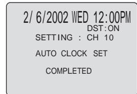
If **AUTO CLOCK SET IS INCOMPLETE** screen appears, set the clock using **MANUAL CLOCK SET** procedure on next page.
