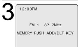
1) Press **CH ▲▼** to select the desired radio station. (Each press changes frequency 200 KHz.)
