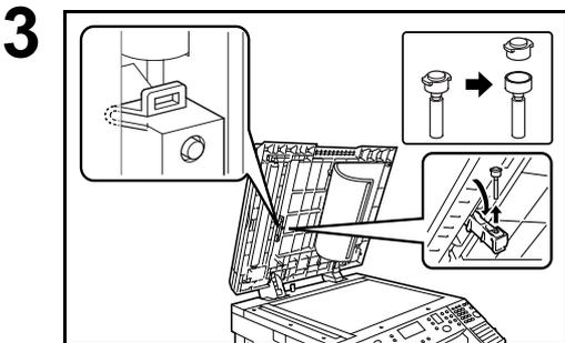
1. Remove by pulling the Stamp Assembly upward.
