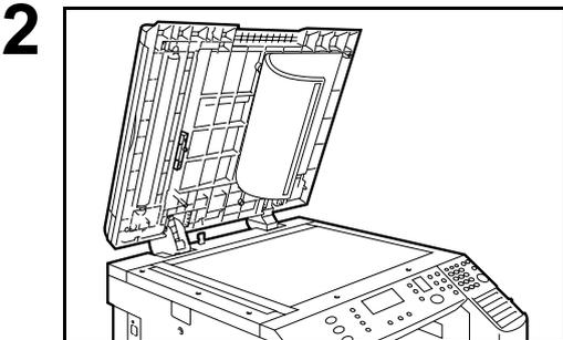
Peel down the Scanning Pad slightly from the left side to expose the Stamp Assembly as illustrated.
