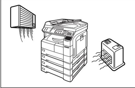
Do not install the machine near heating or an air conditioning unit.
