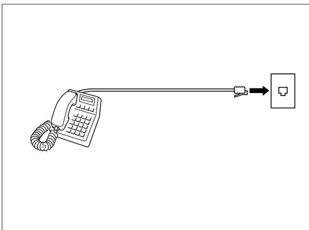
Plug a different regular telephone into the same telephone jack.
