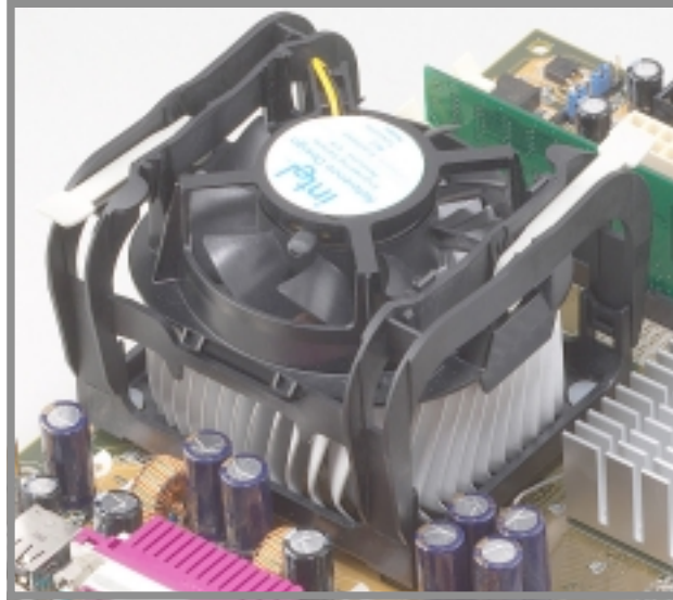
Figure 2-11 Fan and Retention Mechanism Installed and Locked
