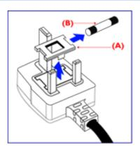
pin plug fitted in its place.
