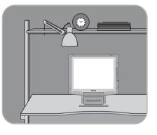
DesXcape 150DM can be used as a desktop monitor when it is on the base station with the base station connected to your computer. In this setup, the AC power adaptor connected to the base station powers DesXcape 150DM while the computer transmits display signals to DesXcape 150DM through a video cable (a VGA cable or a DVI cable). With the power and display signals, DesXcape 150DM acts exactly like a 15" LCD monitor for your computer.
