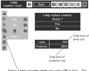
Select Lamp counter reset and press OK button. The message "Lamp replace counter reset?" is displayed.
