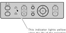
This indicator lights yellow when the life of the projection lamp draws to an end. Replace the Projection Lamp with a new one promptly.
