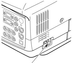
Connect AC power cord (supplied) to the projector. The AC outlet must be near the projector and easily accessible.
