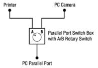
In this way, the switch box enables you to connect both the Philips PCA635VC and a printer (or Zip drive) to ONE parallel port. Any standard mechanical switch box from any computer store will work. DO NOT USE an electronic switch box.
