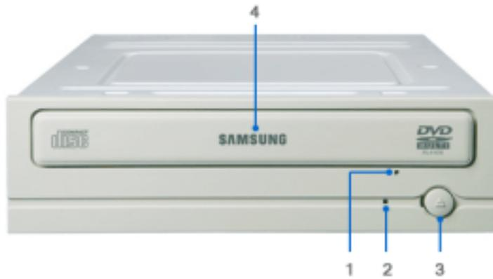
1. Emergency eject hole. (if the compartment does not open when you press the Eject button, power off the computer, insert a pin or unfolded paper clip in the hole and push firmly)
