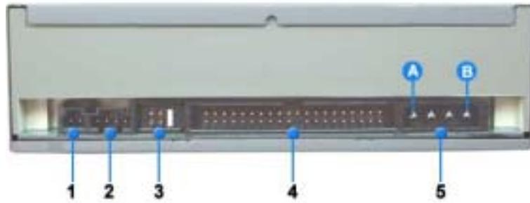
1. Two-pin digital audio output terminal for use with a sound or MPEG card supporting digital audio features.
