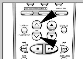
*The Picture Adjustment feature allows you to adjust the alignment manually to obtain the best possible picture.*
