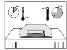
Do NOT expose the DVD-VCR to extreme temperature conditions (below 5°C and above 40°C) or to extreme humidity conditions (less than 10% and more than 75%).
