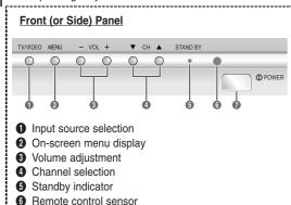
You can use the buttons to switch the TV on when it is in standby mode depending on the model.
