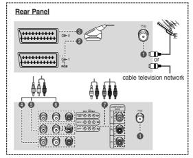
Whenever you connect an audio or video system to your television, ensure that all elements are switched off. Please be sure to match the color coded input terminals and cable jacks.
