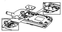
4. Hold the SIM card in position and rotate the holder in the direction of the arrow to lock the SIM card into place.
