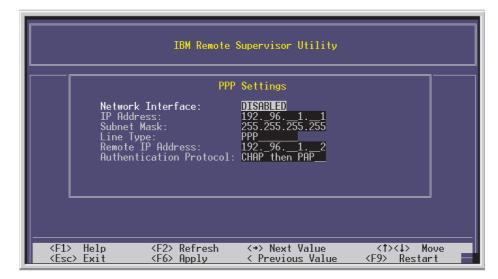
Figure 7. Ethernet Settings window setting up point-to-point protocol
