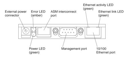
Figure 3. Remote Supervisor Adapter
