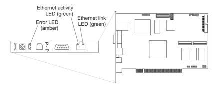
Figure 4. Ethernet LEDs locations on the Remote Supervisor Adapter
