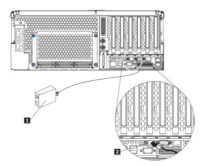
Figure 8. Connecting an ASM Interconnect module to an SmartServer 370
