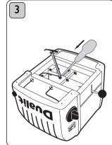
Unplug and place toaster on L a soft cloth. Remove crumb ra tray and unscrew feet s to remove the base plate.
