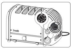
Set the selector switch so **ALL** the slots are active, with **NO** bread in the slots, turn the timer all the way round and let it run back to the off position.
