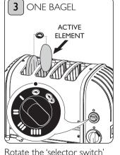
anti-clockwise to the one bagel symbol. Only the second element from the left will heat up.
