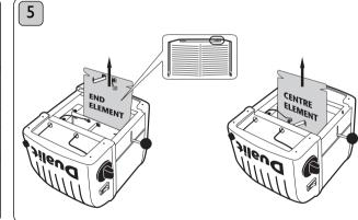
Bend brass links and wires away from the element. Remove element. To re-assemble, reverse procedure ensuring wires and parts are correctly positioned. Ensure new element is marked the same as the one removed and is seated correctly in the channels either side. PAT test before use.
