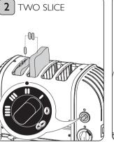
Rotate to the two slice indicator. The first two slots from the left will toast on both sides.
