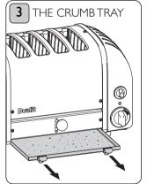
Empty the 'crumb tray' on a regular basis. Daily if being used in a commercial kitchen.
