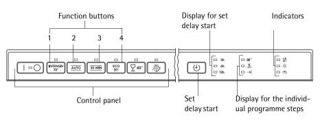
The **control panel** consists of the ON/OFF button III and the programme buttons with LED displays.
