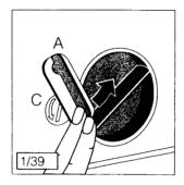
Turn rotary control for emergency drain (A) in clockwise direction.
