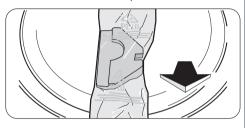
3. Remove foil hose and polystyrene padding from the machine.
