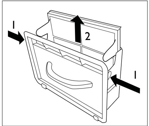
3. Clean the inside of the door, the fluff filter chamber and the rubber seals of fluff.
