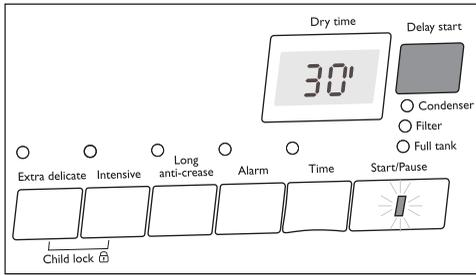
**i** With the *Delay start* button, you can delay the start of a programme by between 30 minutes (30') and a maximum of 20 hours (20h).
