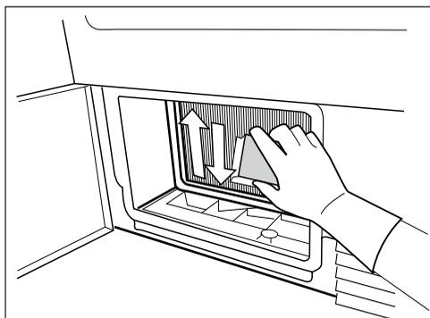
**i** The fluff can be removed more easily if it is first dampened e. g. with a laundry dampener. It is best to use a vacuum cleaner for this purpose.
