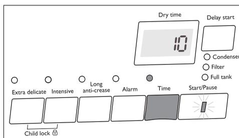
2. Press the *Time* button repeatedly until the desired programme duration is shown in the display, e.g. 20 for a programme of 20 minutes.
