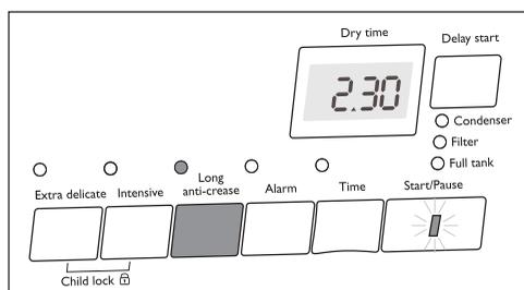
If this additional function is selected, the anti-crease phase at the end of the drying cycle is lengthened by 60 minutes. The laundry can be removed at any time during the anti-crease phase.
