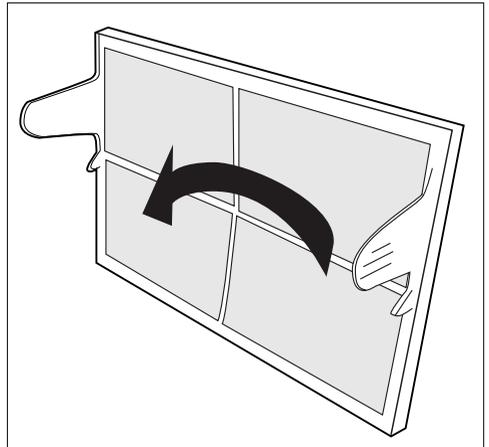
5. To clean the fluff filter: Remove the filter from the filter housing. To do this, press the pressure points on the sides and pull the filter frame up and out of the housing.
