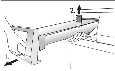
2. Pour the condensed water out into a basin or similar receptacle.
