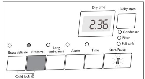
2. Press the *Intensive* button - the LED above is on.
