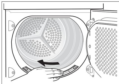
3. After a period of time, a patina due to detergent residue on laundry forms on the filters. When this occurs, clean the filters with warm water using a brush. Remove the filter from the door pulling it out. (It can be positioned with the locating spur facing to the left or to the right).
