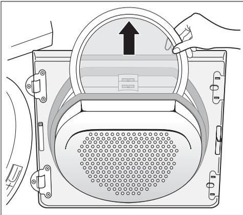
9. Press both journals of the large mesh filter into the brackets on the loading door until they snap into place.
