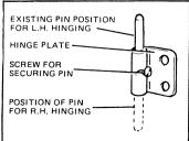
upright. Repeat procedure for bottom hinge. Replace blanking screws in left hand hinge positions in oven. Invert glass door and rehang in new position.
