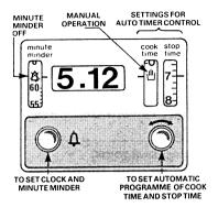
This timer will automatically switch the oven on and off to the selected times. It also includes a clock and minute minder.
